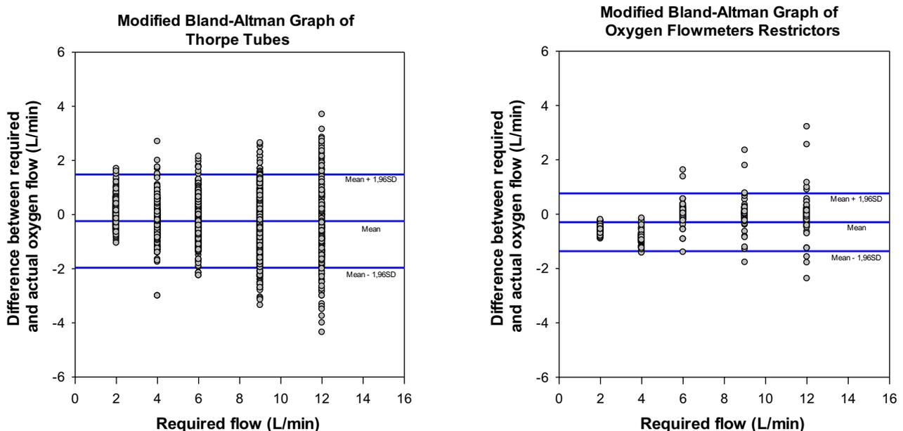
**Fig. 2** Modified Bland Altman analysis of the agreement between required flow and the actual flow for Thorpe tubes (n=476) and oxygen flow restrictors (n=96) at 2, 4, 6, 9 or 12 L/min oxygen flow
