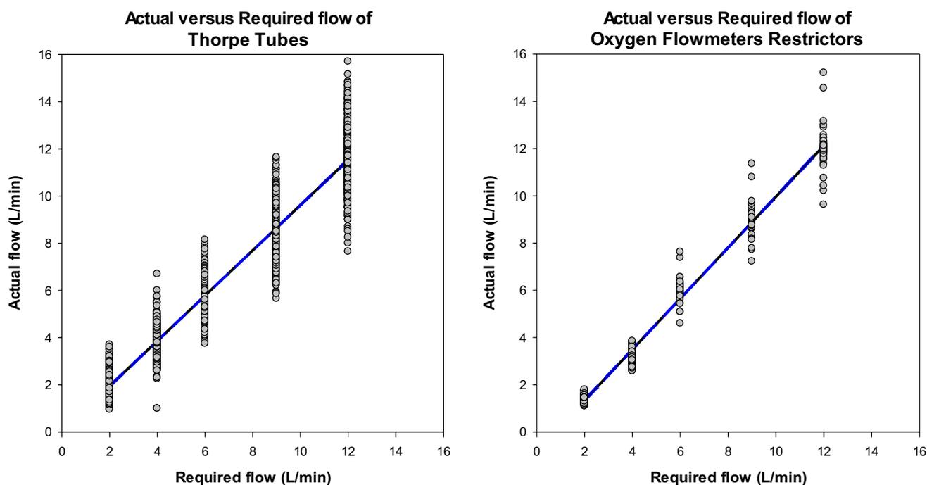
**Fig. 1** Linear regression analysis and scatter plot distribution between required flow and the actual flow of Thorpe tubes (n=476) and oxygen flow restrictors (n=96) at 2, 4, 6, 9 or 12 L/min oxygen flow rates
